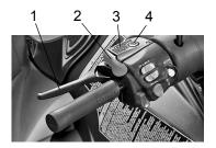
To engage the lock, squeeze the brake lever tightly and push forward on the lock. Hold the lock forward while releasing the brake lever.
